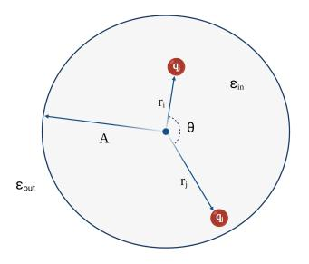
• This model is spherically symmetric, describing several charges embedded in a dielectric with low permittivity  $\varepsilon_{in}$  which is surrounded by a different dielectric with higher permittivity  $\varepsilon_{out}$  • For such a discrete distributed charge system, we can rewrite **Poisson** equation with **Green function**:
