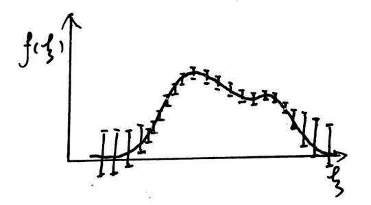
In simulation, PDF can be derived from histogram on collective variables. However, the estimation on the rare events is accompanied with high statistical error • Simulation with bias potential:
